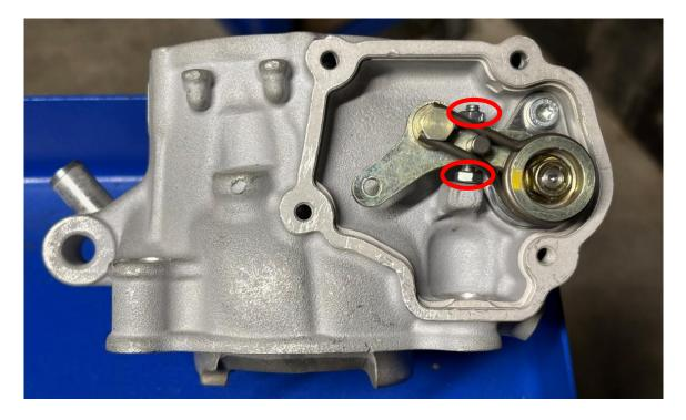
Use a depth gauge and adjust the end stop with the following values:
