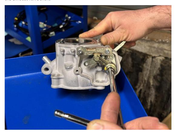
At this point, you have set the all open position, now it remains to adjust the end stop with the valve closed.
